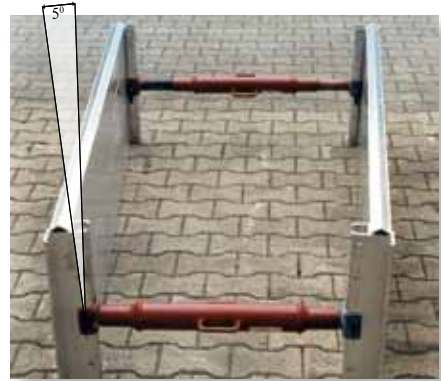
The struts allow the sides to be inclined at an angle of up to 5°.
